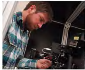
Brandon Scott, Ph.D., a postdoctoral researcher in Nanoscience and Nanoeengineering at SD Mines, adjusts part of the Lattice Light Sheet Microscope (LLSM) used to make dynamic 3D movies showing the inner workings of living cells.
