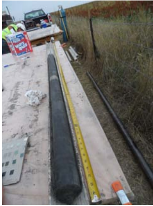
Bentonite in the Pierre Shale
