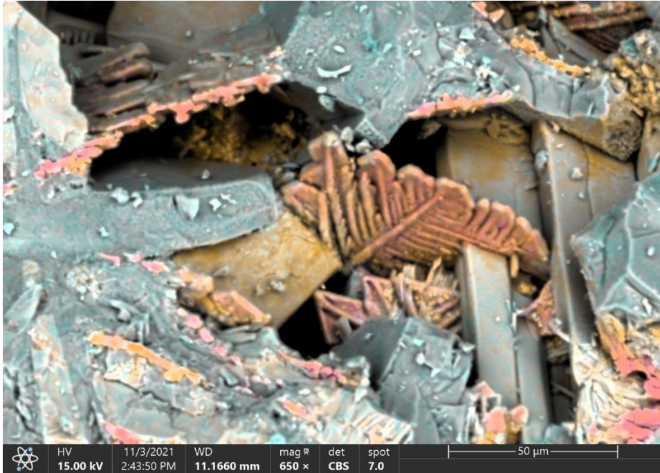
Uncoated sample of Icelandic basalt showing dendritic ilmenite grains (image by Erica Cung, GGE MS student).
