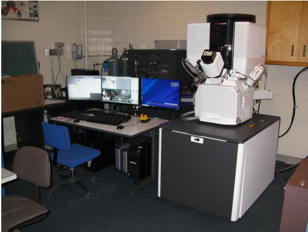
Thermo Fisher Scientific Helios 5 CX FIB-SEM with Energy Dispersive Spectroscopy and Electron Backscatter Diffraction capabilities
