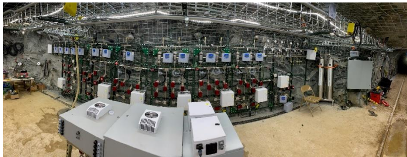
The panoramic, distorted view on the left shows the entirety of the packer control and fluid monitoring systems, whereas a non-distorted view of the drift is seen on the right.
