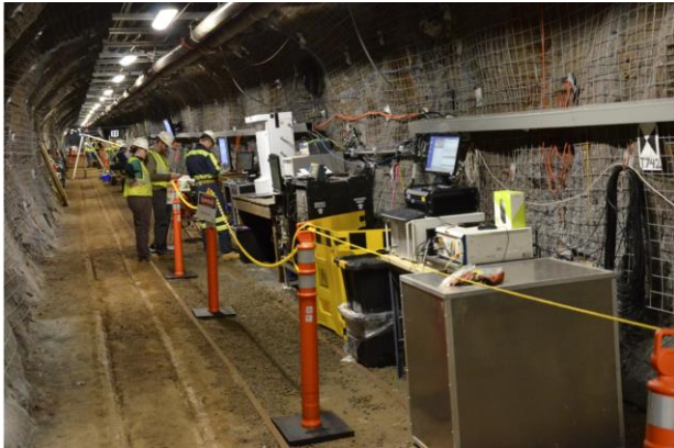
Figure 2. Pumping and monitoring instrumentation at the EGS Collab Test Bed 1 Location on the 4850 Level.
