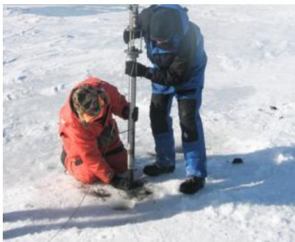
Sampling lake sediment through ice in eastern SD during January 2009.
