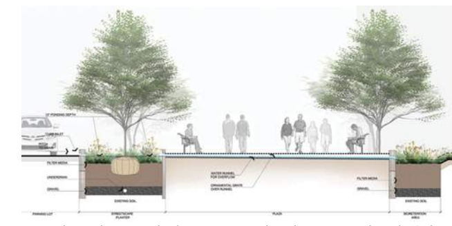
Section showing low impact development practices through an active travel corridor. (online photo)
